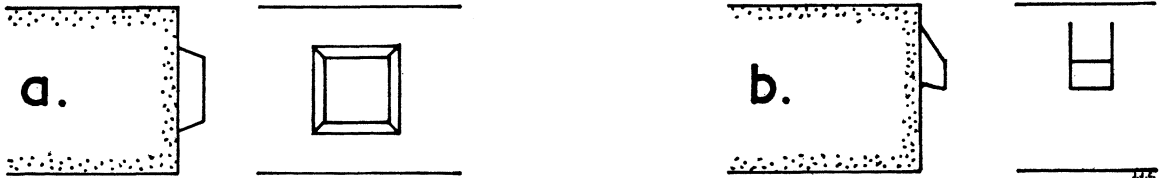
FIG. 5.—Shape and position of projecting bosses: a. typical example as found. b. hypothetical example suitable for use with a loop of rope.
